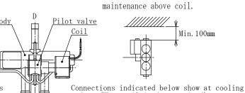
(When coil is de-energized) D connection : Discharge E connection : Evaporator S connection : Suction
