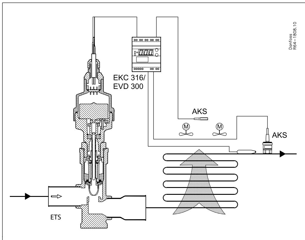
The ETS valves operate modulating by electronically controlled activation of the AST stepper motor. The motor is a type 2-phase bi-polar, which stays in position, unless power pulses from a driver initiate the two discrete sets of motor stator windings for rotation in either directions.
