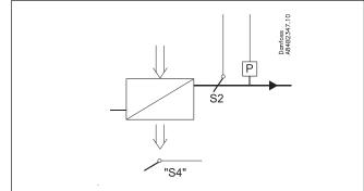
The S4 and T0 temperatures also form part of an inner loop regulation.
