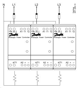
Max. load at: 400 V ACI 30-1 + ECI 30-1 20.7 kW ACI 50-1 + ECI 50-1 34.1 kW
