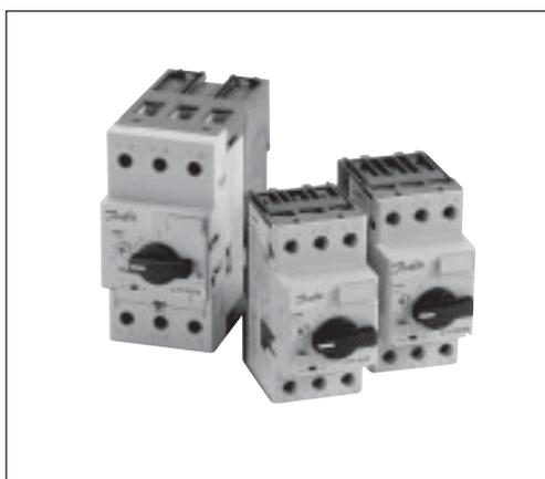
Circuit breakers for overload- and short circuit protection of transformer applications cover the current range 0.1 – 32A. The circuit breaker breaks at a very high electromagnetic trip current. The product program is split up in three product sizes. The smallest size is called CTI 16T. It consists of 11 code numbers and covers the current range from 0.1 – 16A. The next size is
