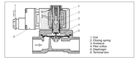
Proportional regulation of the opening and closing of the EV260B valves is achieved through stepless regulation of the coil current and thus of the pulling force of the solenoid coil.
