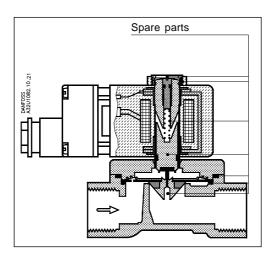
The spare parts kit comprises e.g. a locking button and nut for the coil, armature with valve plate, spring, O-rings and diaphragm.
