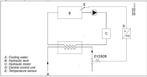
To control viscosity and thus friction, it is important to keep a constant oil temperature in hydraulic motor (C). Cooling is therefore often required.
