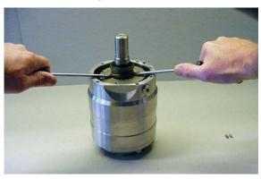
6. Remove guide pin from housing and the two guide pins from swash plate.
