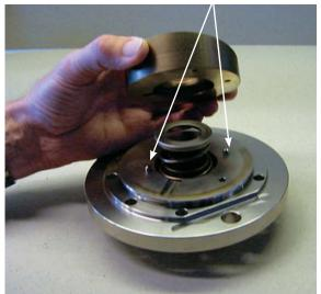
18. Press swash plate against front flange and screw tools together.
