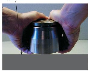
9. Mount cylinder barrel in housing.
