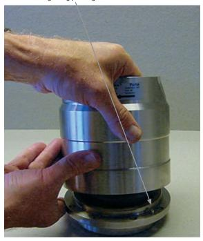
Place housing and port flange near table edge and mount screws from below.
