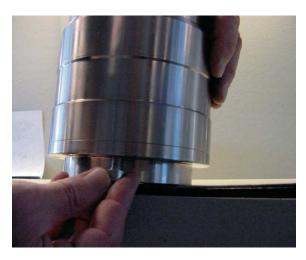
7. Mount thrust plate with sealings on cylinder barrel.
