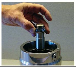
11. Mount retaining plate (smallest centre diameter pointing upwards).
