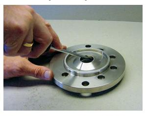
18. The ceramic ring removed from the front flange.
