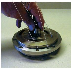
4. Mount valve plate in its right position using pin as guide.
