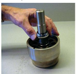
16. Remove thrust plate using two screwdrivers.
