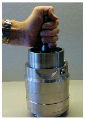
10. Slide retaining ball (smallest diameter pointing upwards) down the shaft.
