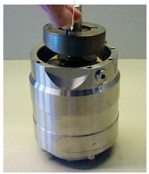
8. Remove cylinder barrel from housing.
