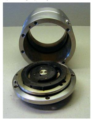
11. Remove valve plate from port flange.
