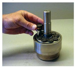
14. Remove retaining plate.
