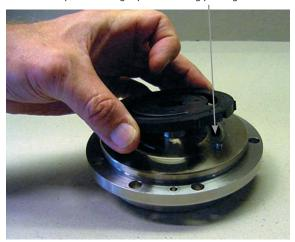
5. Mount housing using pin as guide.
