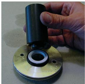
17. Mount the washer with the edge pointing upwards.
