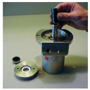
20. Wet the shaft seal and slide it over the bush.
