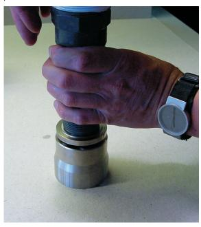
Check that the gap between the cylinder barrel and the thrust plate is 1.5-2.5 mm.
