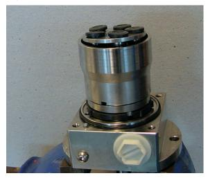
12. Mount the pump housing using the pin as guide.
