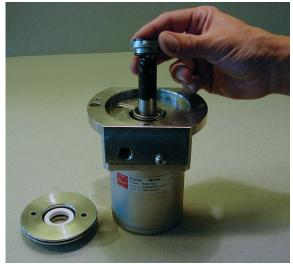
21. Use the shaft seal tool when pressing the shaft seal downwards.
