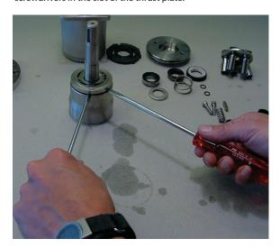
12. Remove the thrust plate.
