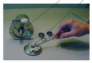
6. Unscrew the four screws for the housing.
