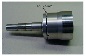
8. Mount the cylinder barrel in the flange.
