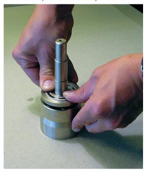
6. Press the thrust plate into the cylinder barrel using a piece of plastic.
