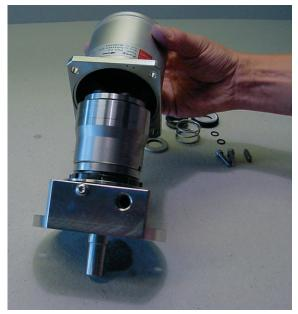
8. Remove the cylinder barrel.
