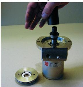
22. Press the shaft seal in position.
