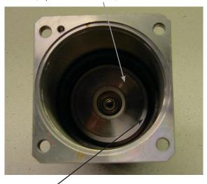
2. Check the bearing (the black part) for large wear grooves (not critical).
