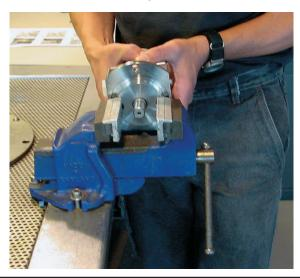
4. Remove the shaft seal using two screwdrivers.
