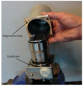
13. Press the housing down by hand and insert the screws.
