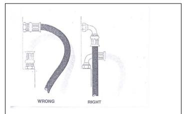
Elbows and adaptors should be used to relieve strain on the assembly and to provide well-organized installations to facilitate access for inspection and maintenance.
