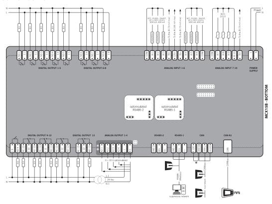
\*NOTE: connection has to be made on the first and last local network units, make the connection as close as possible to the connector
