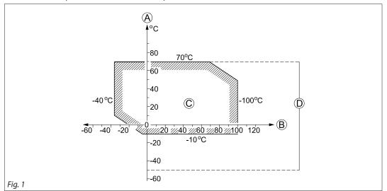
A: Ambient temperature B: Temperature and medium C: Operating range
