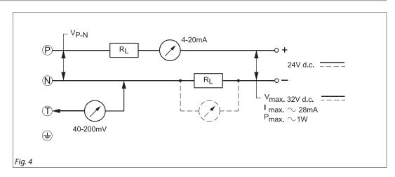
The transmitter has a wiring diagram, see fig. 4. Terminals P (positive) and N (negative) are connection terminals for the supply voltage.
