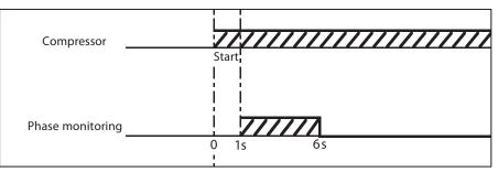
The phase sequencing and phase loss monitoring functions are active during a 5-sec window 1 sec after compressor start-up (power on L1-L2-L3).
