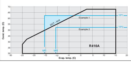
Example 1 (R410A, SH = 11 K) LP switch setting: LP1 = 3.3 bar (g) (-15.5°C) HP switch setting: HP1 = 38 bar (g) (62°C) Risk of operation beyond the application envelope. DGT protection required. **Example 2** (R410A, SH = 11 K) LP switch setting: LP2 = 4.6 bar (g) (-10.5°C) HP switch setting: HP2 = 31 bar (g) (52°C) No risk of operation beyond the application envelope. No DGT protection required.
