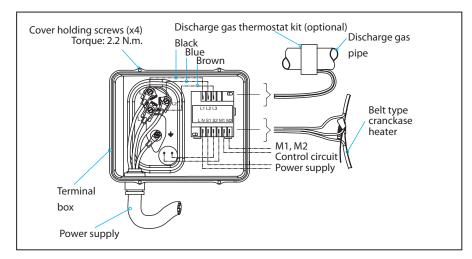
The motor protection module comes preinstalled within the terminal box. Phase sequence protection connections and thermistor connections are pre-wired. The module must be connected to a power supply of the appropriate voltage. The module terminals are 6.3-mm size Faston type.
