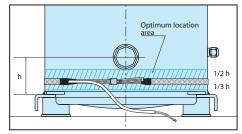
The belt-type crankcase heaters are designed to protect the compressor against off-cycle migration of refrige-rant.
