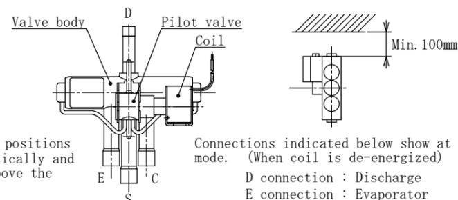
Connections indicated below show at cooling mode. (When coil is de-energized)
