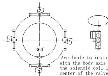
Available to install in any positions with the body axis held vertically and the solenoid coil located above the center of the valve. 360°
