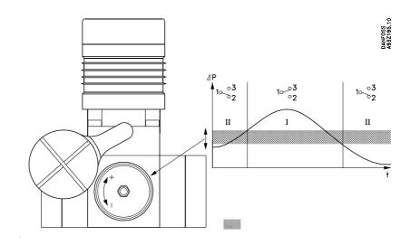
One turn of the MBC setting-screw is approx. equal to 7% of FS (max. setting range)
