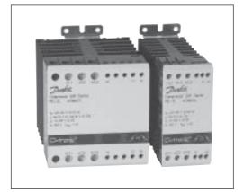
The MCI compressor soft starters are designed for soft starting of 3 phase compressors. During start the MCI will gradually increase the voltage to the motor until it reaches full line voltage.
