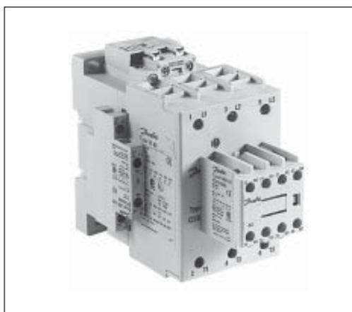
Contactors CI 61, CI 73 and CI 86 switch powers of up to 30 kW, 37 kW and 45 kW respectively under 3 x 380 V AC-3 loads. Overload relays TI 80 and TI 86 together with current rail set 037H0108 fit on the three contactor types.
