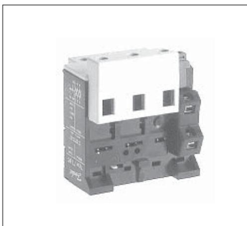
Thermal overload relays TI 80-86 are used with contactors type CI 61, CI 73 and CI 86 to give overload protection of squirrel-cage motors of 30 kW to 45 kW. The relays trip under asymmetric load, i.e. accelerated release if phase drop-out occurs.
