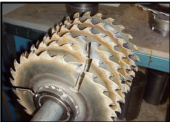
Insufficiently or non-lubricated system in use
