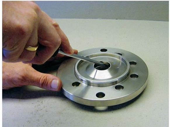
18. The ceramic ring removed from the front flange.
