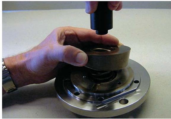
15. Mount the shaft seal (carbon surface pointing downwards), the spring, and the washer (edge pointing downwards) by sliding them over the tool.
