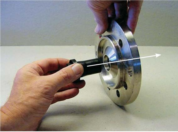
17. Press the swash plate against the flange and screw the tools together.
