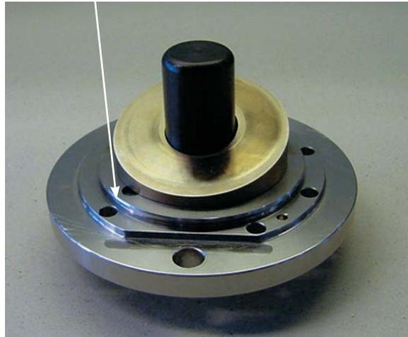
16. Mount the swash plate on the front flange using the pins as guide.
