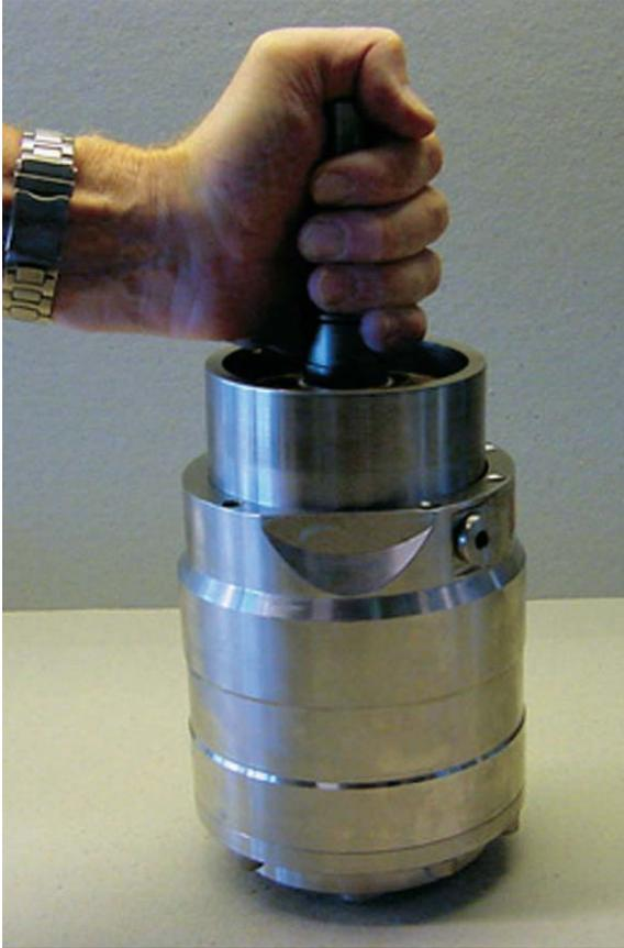
10. Mount the retaining plate (smallest centre diameter pointing upwards).
