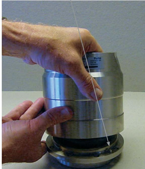
6. Mount the thrust plate with sealings on the cylinder barrel.
