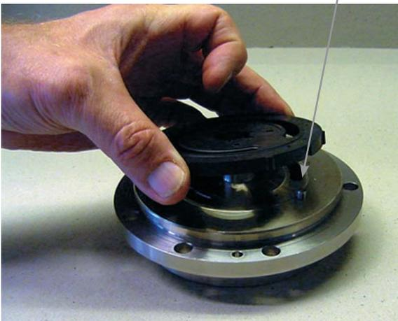
5. Mount the housing using the pin as guide.
