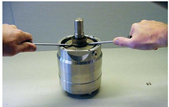
6. Remove the guide pin from the housing and the two guide pins from the swash plate.
