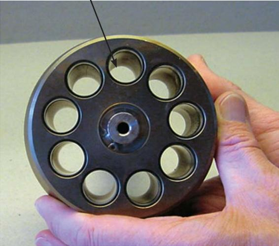
3. Ensure that the pistons can move freely in the bushings.
