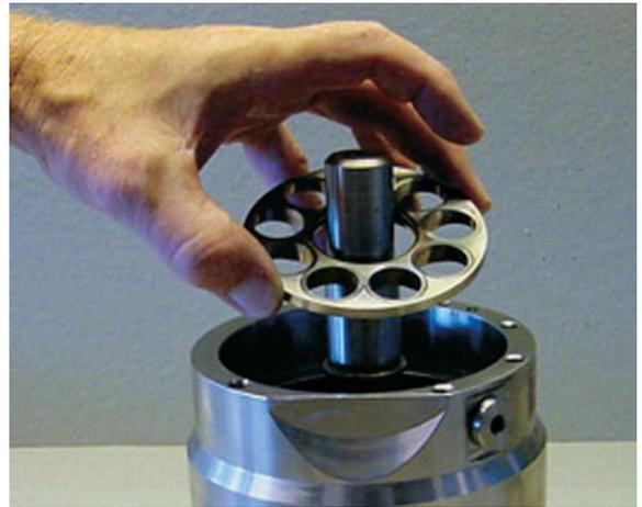
9. Slide the retaining ball (smallest diameter pointing upwards) down the shaft.
