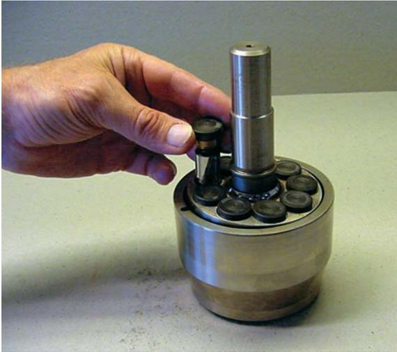
14. Remove the retaining plate.
