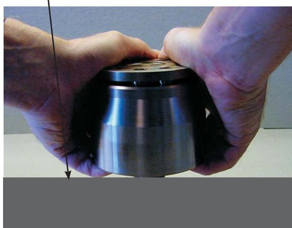
8. Mount the cylinder barrel in the housing.
