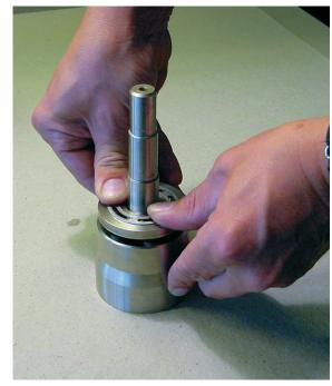
6. Press the thrust plate into the cylinder barrel using a piece of plastic.
