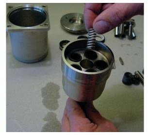
13. Loosen the thrust plate using two screwdrivers. Place one of the screwdrivers in the slot of the thrust plate.
