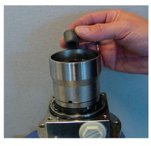
11. Mount the retainer guide on the spring guide.
