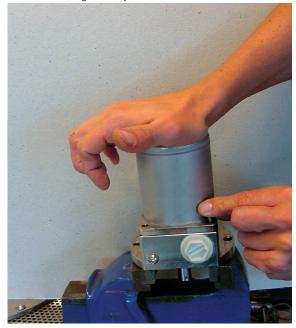
17. Tighten the screws to a torque of 22 Nm.
