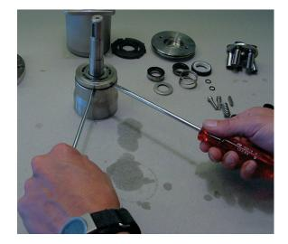
14. Remove the thrust plate.
