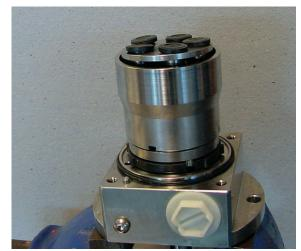
15. Mount the pump housing using the pin as guide.
