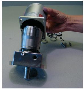
8. Remove the cylinder barrel.
