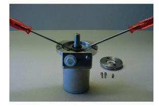
5. Remove the two small O-rings from the flange. Remove the seal from the front cover using a screwdriver.
