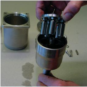
10. Remove the retaining guide.
