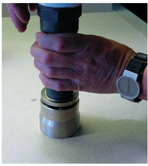
7. Check that the gap between the cylinder barrel and the thrust plate is 1.5-2.5 mm.
