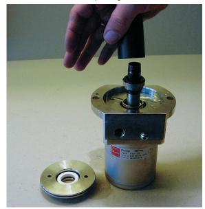
25. Press the shaft seal in position.
