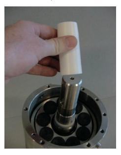
9. Thoroughly wet the torpedo, shaft and replacement shaft seal with plenty of soap. **Do not use silicone grease.**
