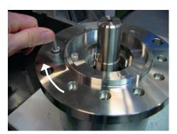
15. Remove the ceramic ring from the seal retaining ring.
