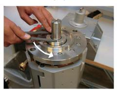
2. Unscrew the 8 screws in the mounting flange.
