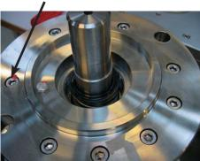
3. Carefully remove the flange from the casing.
