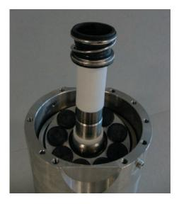
Use the plastic assembly tool provided, large diameter pointing downwards, to press the seal home against the shoulder of the spacer.
