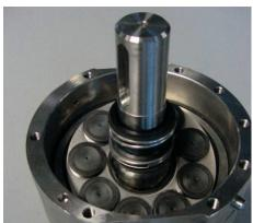
12. Remove the old O-ring and fit the new O-ring on the adapter.
