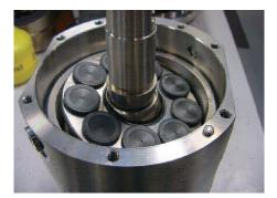
7. Scrap the old spacer (if black) and place the new white spacer on top of the retaining ball.
