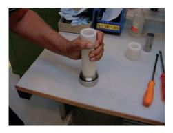
Make sure the face with the rubber seal is positioned against the shoulder in the retaining ring (see drawing on last page).
