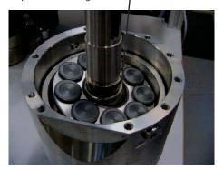
8. Fit the hollow bush (torpedo) onto the shaft.
