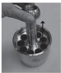
8. Carefully remove the valve plate assembly using a screwdriver.
