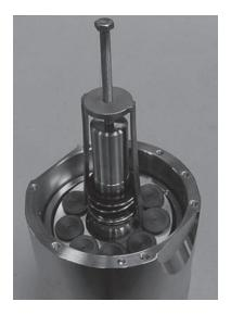
6. Remove the whole cylinder barrel and carefully place it on a suitable clean surface.
