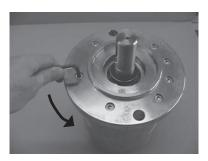
3. Carefully remove the mounting flange from the housing.
