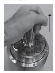
7. Remove the pistons, retaining plate, distance ring and retaining ball from the cylinder barrel.
