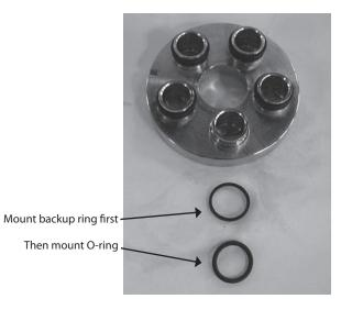
11. Wet the O-rings and back-up rings with clean (filtered) soapwater.
