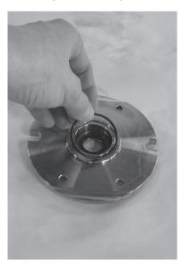
20. Lubricate the threads on the 4 screws with grease and screw them into the pump and tighten by hand. Use Molykote<sup>®</sup> D paste from Dow Corning or Klüber UH1 84-201 from Klüber lubrication.
