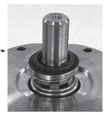
19. Replace the O-ring on the SAE flange.
