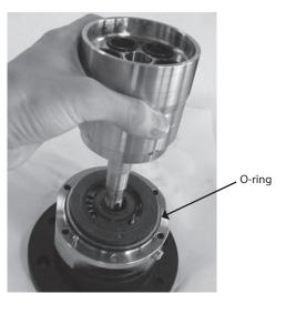
15. Position the new spring, new spring guide, new retaining ball, new retainer guide and new pistons.
