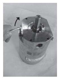
18. Mount the new shaft seal following the instructions in "Shaft Seal - APP1.5-2.5" (521B0737).
