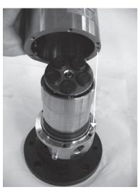
17. Hold the pump together and carefully turn it over to rest on the housing. To prevent seizing-up, lubricate the threads on the 2 screws and screw them into the port flange and the housing. Use Molykote® D paste from Dow Corning or Klüber UH1 84-201 from Klüber lubrication. Tighten the 2 flange screws to a torque of 12 +1 Nm.
