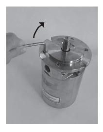
21. Tighten the screws to a torque of  $12 \pm 3$  Nm.
