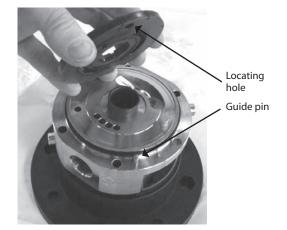
IMPORTANT: Make sure that the guide pin is located in the locating hole in the port plate.
