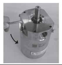
Carefully turn the whole pump over so that the shaft is facing down. Support the pump in a suitable hollow base so that the pump is not supported by the shaft.
