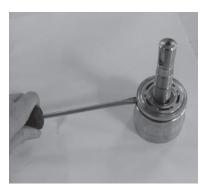
Replace the O-rings and the back-up rings on the valve plate. 10. Mount the new back-up rings on the new valve plate first and then mount the new O-rings.
