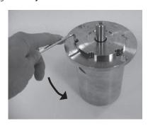
Wet the shaft and shaft seal with clean (filtered) soap-water.
