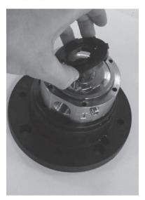
Gently lever the valve plate assembly free with the aid of a 9. screw-driver.
