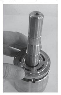
13. Position the new port plate over the guide pin.
