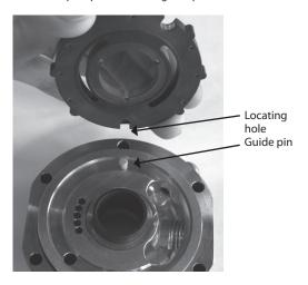
IMPORTANT: Make sure that the guide pin is located in the locating hole in the port plate.
