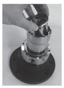
7. Remove the cylinder barrel.
