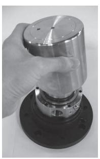
Remove the pistons, retaining plate, retaining ball, spring guide 8. 6. and spring from the cylinder barrel.
