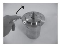
21. Tighten the screws to a torque of  $8 \pm 3$  Nm.
