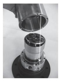
17. Hold the pump together and carefully turn it over to rest on the housing. To prevent seizing-up, lubricate the threads on the 2 screws and screw them into the port flange and the housing. Use Molykote® D paste from Dow Corning or Klüber UH1 84-201 from Klüber lubrication. Tighten the 2 flange screws to a torque of 8 +1 Nm.
