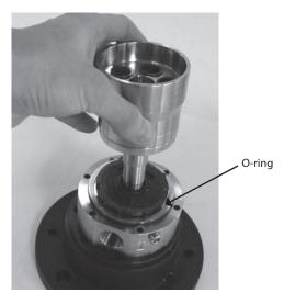
15. Position the new spring, new spring guide, new retaining ball, new retainer guide and new pistons.
