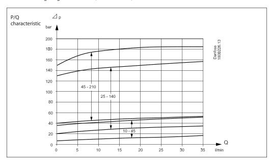
Max. flow: 60 l/min
