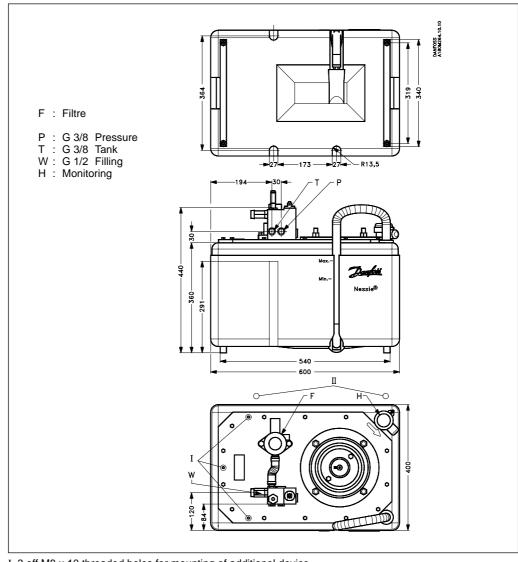
I 3 off M8 x 10 threaded holes for mounting of additionel device. II 6 off M10 x 8 threaded inserts in tank body for mounting of additional device.
