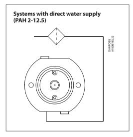
In order to eliminate the risk of cavitation, a positive inlet pressure is always to be maintained.
