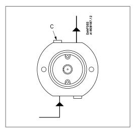
Before starting the pump, the top bleeding plug "C" is loosened. When water appears from the bleeding plug, the pump is filled with water, and the plug is retightened. Make sure that rotation direction of the pump is correct.
