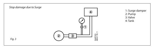
In cases where valves are closed momentarily, surges af a value in excess of that for which the pressure element is designed can occur. To avoid damage to the pressure element, a damping device should
